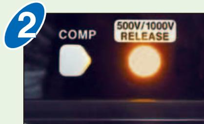
Press the flashing "RELEASE" key.
