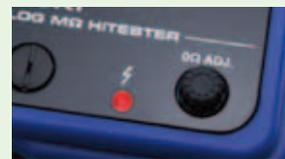
The LIVE CIRCUIT LED will light up in red whenever the voltage exceeds 20V AC between the LINE and EARTH terminals, and when at least 20V DC is still remaining during the auto discharge.
