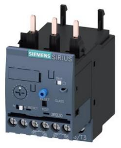
Overload relay 3...12 A Electronic For motor protection Size S0, Class 10E Contactor mounting Main circuit: Screw Auxiliary circuit: Screw Manual-Automatic-Reset
